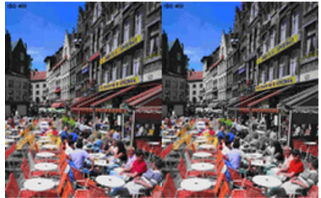
Fig. 6. Spatial Scalability: Decoded images at one-fifth of the original bit-rate. The image on the left is optimized for low resolution viewing and the image on the right is optimized for high resolution viewing. Each image is decoded to the high resolution size of 512 \times 640 pixels, then downsampled, using pixel-averaging, for low resolution viewing at 128 \times 160 pixels. The image on the right is missing color quality for some of the cafe patrons in the middle of the image as well as on the building sides. This is due to the inclusion of high resolution detail, such as sharp edges, which cannot be displayed at low resolution viewing.
